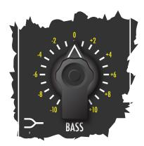
allowing for boost or cut of up to  $\pm$ 10 dB, at fixed frequencies. The Treble control was a peaking bell type, fixed at 10 kHz, while Bass was shelving at 50 Hz.
