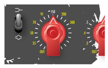
**Note:** Beginning with the TG12345 MK.II desk, the low frequency had a single shelving selection and the presence had eight peaking selections. In the spirit of making the ultimate TG EQ, we reproduced the curves of the shelving and peaking bands so that the treble and bass sections can now use the curves of each. I.e. You may now peak or shelf on the bottom or top.
