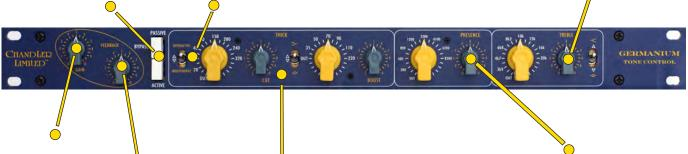
GERMANIUM DRIVE-This controls the input gain of the Germanium amp. The amount of gain from this is related to the Feedback control position.
