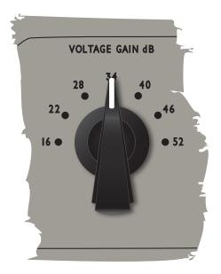
TIP: When gain staging, begin with 'OUTPUT' fully clock-wise, 'FINE GAIN SET' at zero, and set the gain first using the 'VOLTAGE GAIN' control. Once the approximate 'VOLTAGE GAIN' or input gain has been acquired, use the 'FINE GAIN SET' control to adjust for optimum level, and color.
