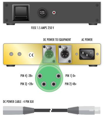
**Note:** Legacy PSU-1 power supplies featured external grounding studs. As of mid 2015, grounding studs have been removed and resistance applied internally.
