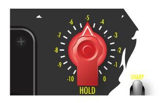
**Note:** The Hold control works independently of level applied to the compressor, i.e. regardless of where the meter needle is placed, the hotter the input signal into the TGI Opto is, the greater the rate of compression be.
