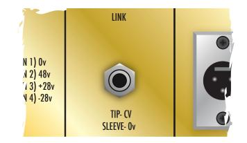
**Note:** When using the TGI Opto independently of a second unit or in mono, be sure to remove any link cable as to not cause undesired influence of one another.
