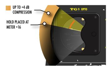
Adjusting the *Hold* control anticlockwise, and placing the meter needle at 0 on the scale will provide up to +20 dB of available compression.
